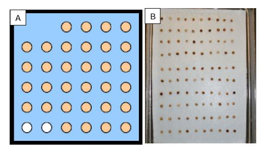
**Fig. 1A.** Drawing (not to scale) representing the layout of 34 spinach seeds on a Steel blue blotter or NP-10 agar medium in a 10 cm x 10 cm Hoffman acrylic box, and **1B.** Photo showing 100 spinach seeds on a blotter paper in a 20 cm x 14 cm acrylic box.
